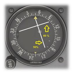
For the virtual glideslope tracking to arm automatically when the pilot initiates APR (Approach) mode, the localizer deflection must be no more than 50% of maximum, the aircraft must be under the glideslope, and the glideslope deflection must be at least 60% of maximum.
