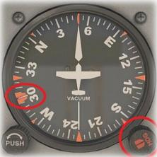
Using the HDG (Heading) bug, manually select the desired intercept course.
