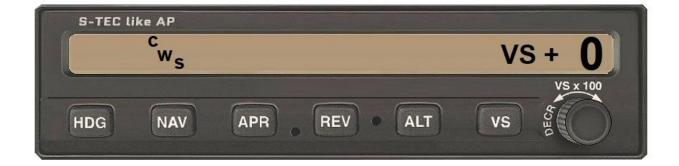
In this mode, the autopilot suspends control of the aileron and trim servos, allowing the pilot to provide the desired input via the control column.
