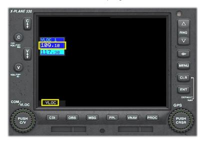
Using your primary navigation radio (in this example the GNS 530), select the desired ILS frequency.
