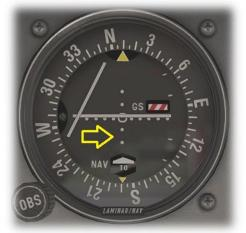
When the Course Deviation Indicator on the VOR instrument is centered, the aircraft is on the desired radial, and the autopilot will maintain that situation.
