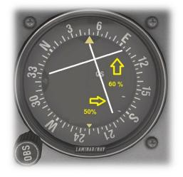
If glideslope tracking does not arm automatically, the pilot may force this to occur manually – after satisfying the 50% / 60% rules for glideslope arming outlined above. Push the ALT button to engage ALTITUDE HOLD and GLIDESLOPE modes concurrently.
